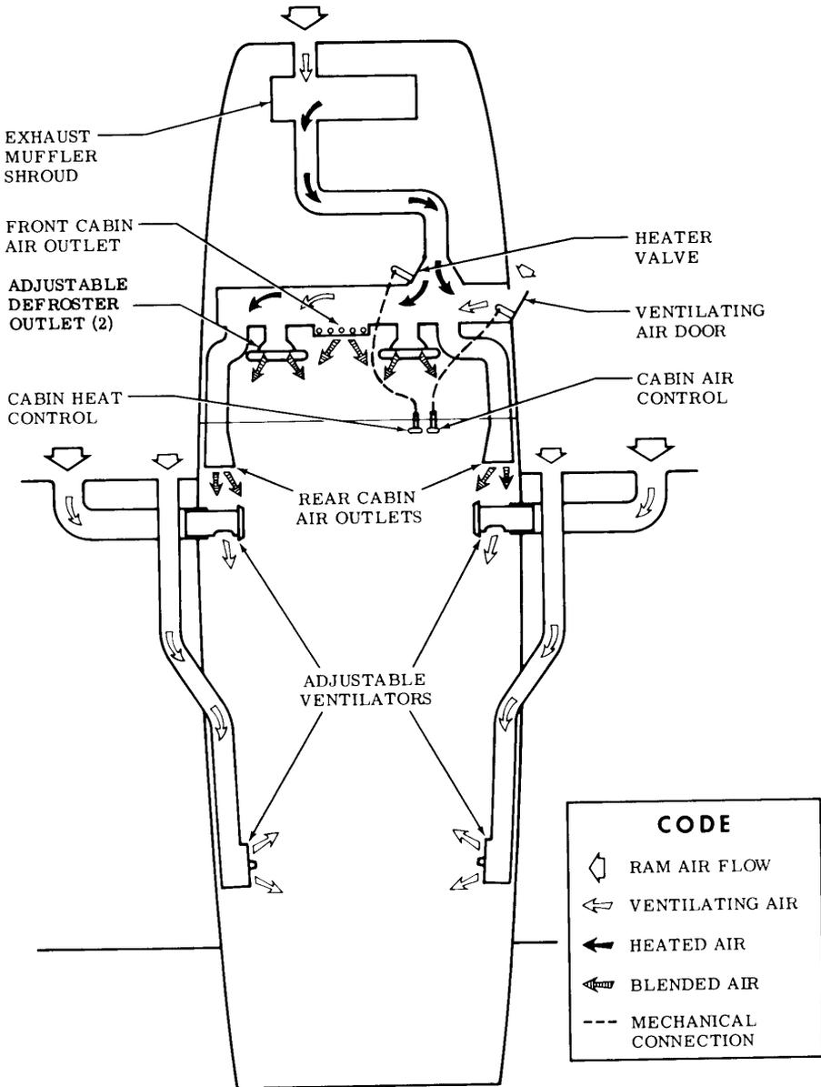
Figure 7-8. Cabin Heating, Ventilating, and Defrosting System
