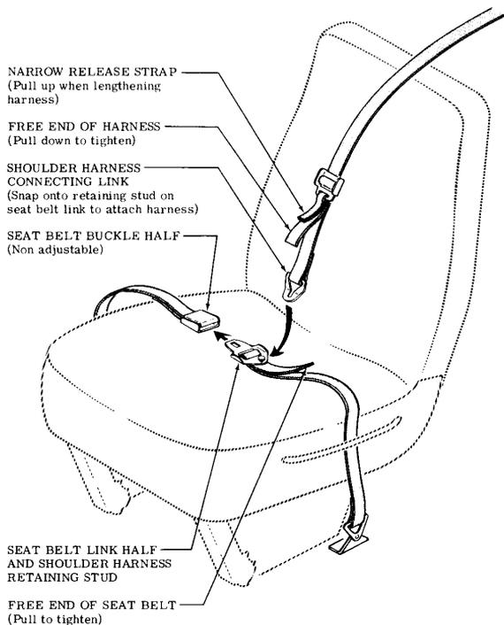
Figure 7-4. Seat Belts and Shoulder Harnesses
